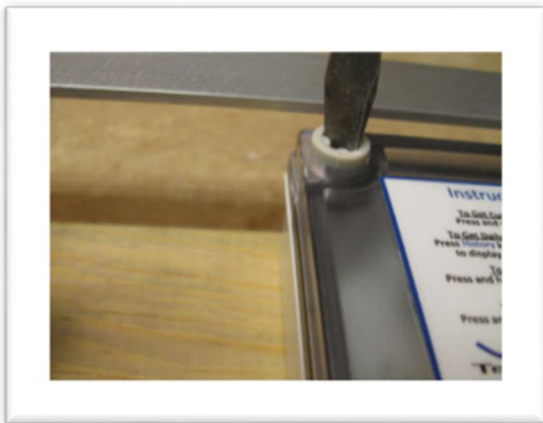
Figure 1: Removing cover screws
